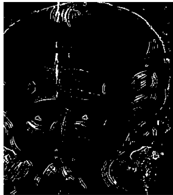
Figure 6: Crack Map after Supervised Classification
